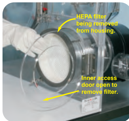
#800-HEPA/S with filter access door open Internal view (When changing filters)
