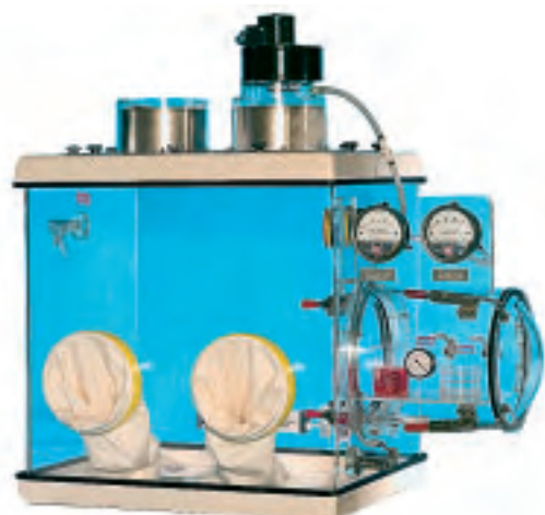
#800-HEPA/D. Open exhaust (double) HEPA filtration system
