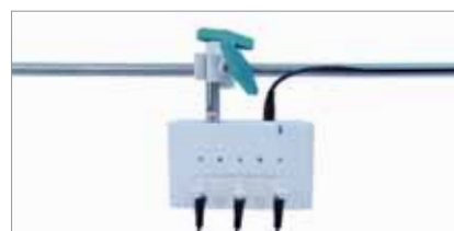
Power divider (5 channels 1) )
