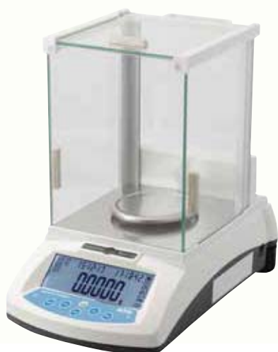
Analytical Balance “WBA-220A” [d] 0.1mg, max.220g
