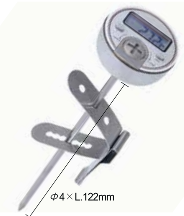
Metal Housing Waterproof(IP67) Thermometer
