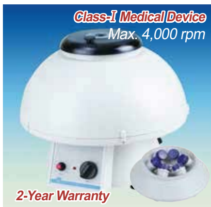
III. “Cef-50.6” for 6 Tubes of 50ml, with 6 Holes Fixed Angle Rotor, 4000rpm
