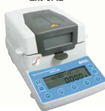
Moisture Analyzer “WBA-110M” [d] 1mg, max.110g
