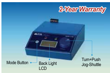
Digital Feedback Temp. Controller “WHM-C10D”
