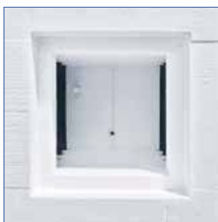
Inner Chamber of Exposed Heating Elements-type
