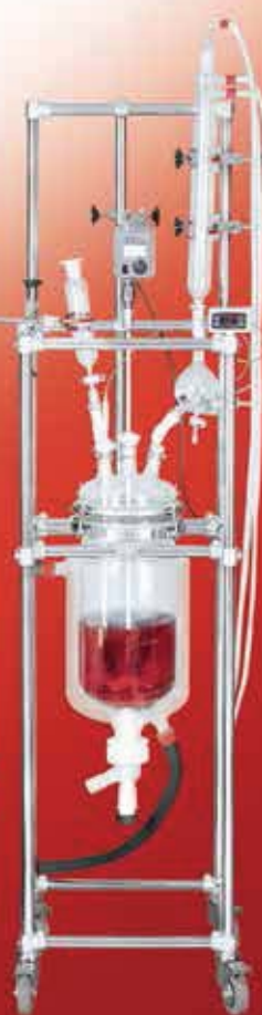
0.5~20 Lit. Suspended-Model III Double-Wall Vessel Good for Economic Operation
