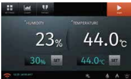
7" Full Touch Screen TFT LCD (Smart-Lab™ Controller)
