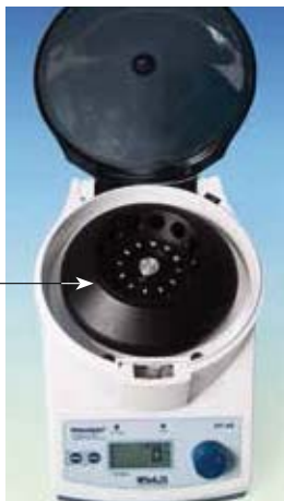
(1) MC Nylon Fixed Angle Rotor for 12×0.2-/0.5-/1.5-/2.0-ml
