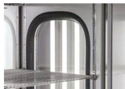
Much light, but not too much heat. These fluorescent lamps are thermally insulated from the test room.
