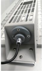
The hot-ball anemometer monitors the wind speed in the working area and exhaust area of the safety cabinet in real time, then compares this with the standard wind speed. The rotating speed of the fan is adjusted through the microprocessor system to maintain the constant wind speed of the safety cabinet.
