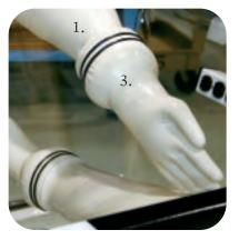
Assembled hand/sleeve set up
