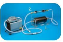
Oxygen trap. Part #2 is the Oxygen indicator (sensor). The accessory is attached only after the initial purge cycles have been completed. It will reduce trace amounts of Oxygen down to about ten (10) ppb. Refer also to Page #41.
