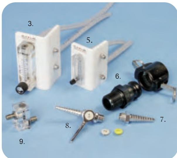
5. **#800-FLOW/D. SMALL FLOW METER** used for smaller chambers and desiccators. Helps regulate gas flow at lower incoming pressures. Kit includes flowmeter, mounting bracket, hoses and ring clips. Range "5-50 SCFH."
