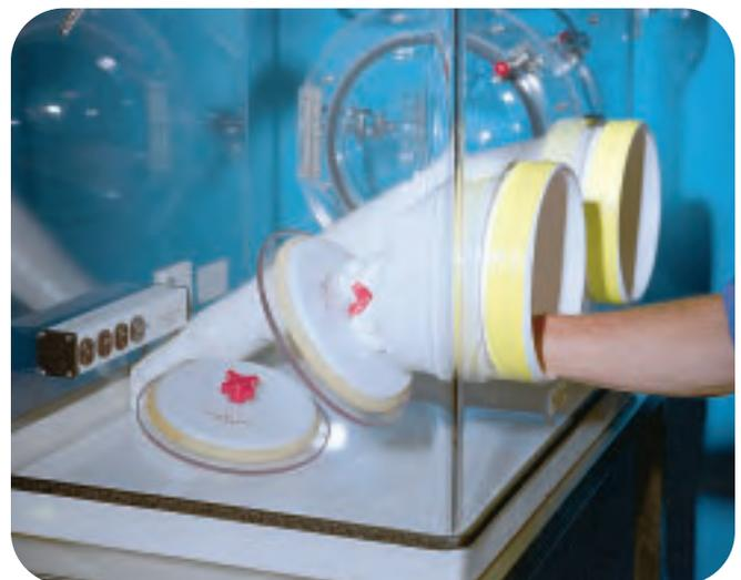
Insert plug into port opening and rotate red knob (tighten) until port is sealed.
