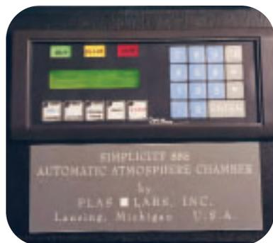
The operator interface continually displays the "PLC" functions and working pressures within the main chamber or transfer chamber. It can also support an additional 4-20 mAmp analog input. These inputs are used to create your own unique atmosphere chamber. Examples are percentage of O<sub>2</sub> analyzer, humidity information, etc.
